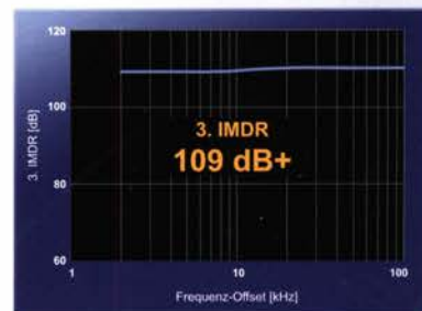
14 MHz Band 3. Intermodulation Dynamic Range (IMDR)
